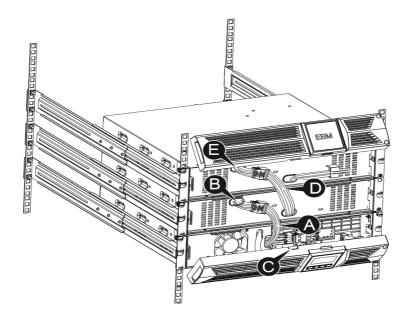
3. Once all of the EBMs have been successfully connected to the UPS and the front panel has been reassembled correctly the UPS needs to be configured to recognise the number of EBMs that have been installed.
