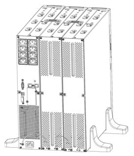
2. Take off the front panel. To do this remove the 2 top screws from the front of the UPS and carefully take out the LCD screen and remove the screw. Finally push inward the small gate on the side of the front panel in order to remove it. This then enables you to connect the battery terminal (A) from the UPS to the EBM terminal (B) shown below. Then connect the battery terminal (D) from the first EBM to the battery terminal (E) of the second EBM. Then users need to reassemble the front panel.
