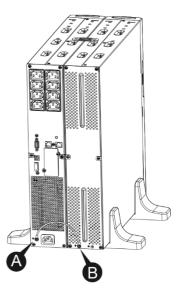
4. Take off the front panel. To do this remove the 2 top screws from the front of the UPS and carefully take out the LCD screen and remove the screw that's behind it. Finally push inward the small gate on the side of the front panel in order to remove it. This then enables you to connect battery terminal (A) from the UPS to the EBM terminal (B) shown below. After doing this reassemble the front panel.
