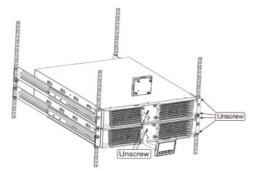
4. Take off the front panel. To do this remove the 2 top screws from the front of the UPS and carefully take out the LCD screen and remove the screw. Finally push inward the small gate on the side of the front panel in order to remove it. This then enables you to connect the battery terminal (A) from the UPS to the EBM terminal (B) shown below.
